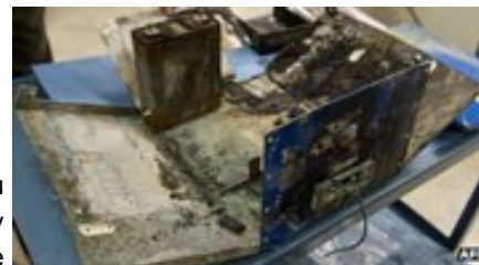
Photograph of Boeing Dreamliner Battery Enclosure after Fire
