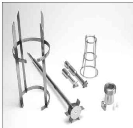
Figure 2 – Internals for the three reactor types studied
